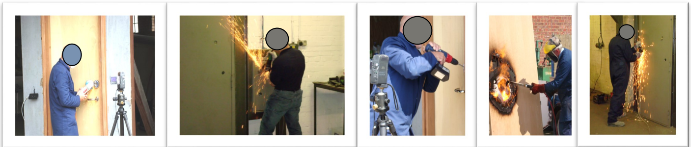
Simulated forced entry tests to BS Standards on Steel and wooden re-enforced doors. Gross attack confirmed
